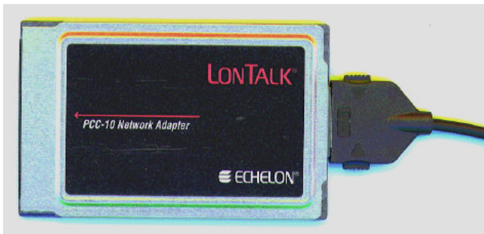
Example of an PCMCIA card from Echelon for use in a notebook
